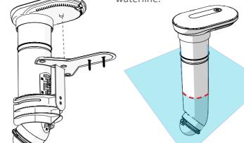
**D.** Mount the docking station using screws and anchors found in the accessories pack, then attach the base plate cover.
