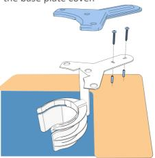
**G.** Insert the pool unit pin in a straight or a rotated docking position and connect to power.
