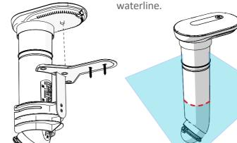
**D.** Mount the docking station using screws and anchors found in the accessories pack, then attach the base plate cover.
